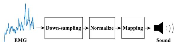
Figure 3: Block diagram of the system.
